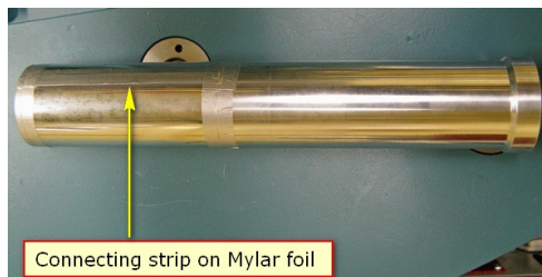
Heat radiation shield (Mylar foil coated with Al)
