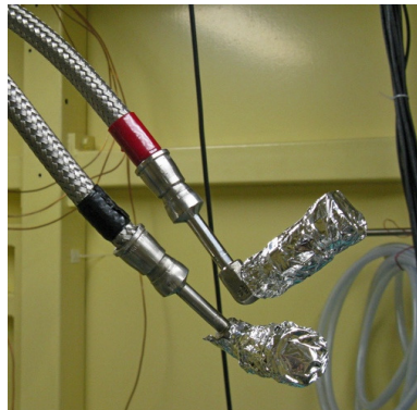
CCR outlet and inlet using the red markers on the tubing to the cryo-head
